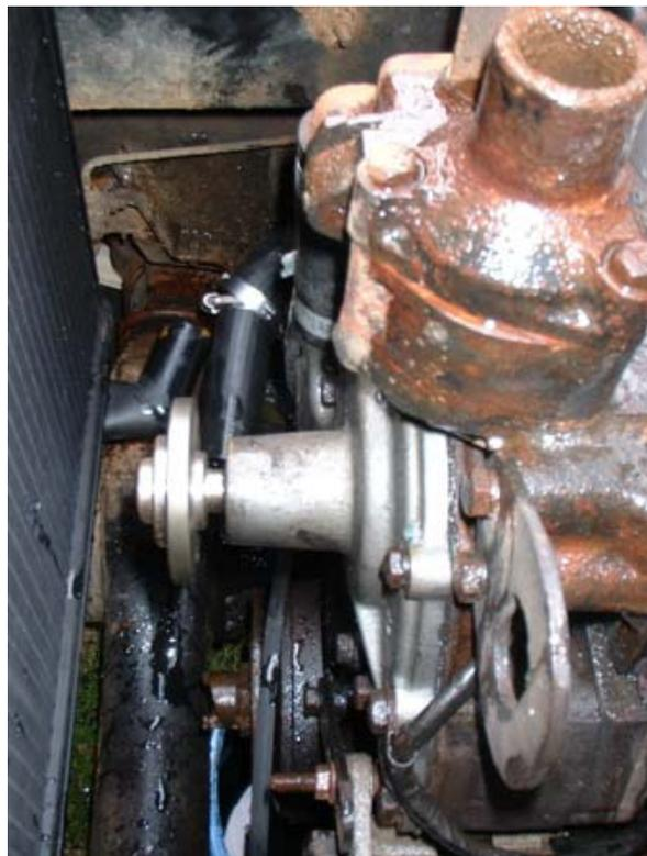
Undo the jubilee clips holding the bypass hose to the pump body and thermostat housing, and then start to remove the bolts holding the pump in position. Military water pumps have 7 bolts, and civilian ones have 9.
