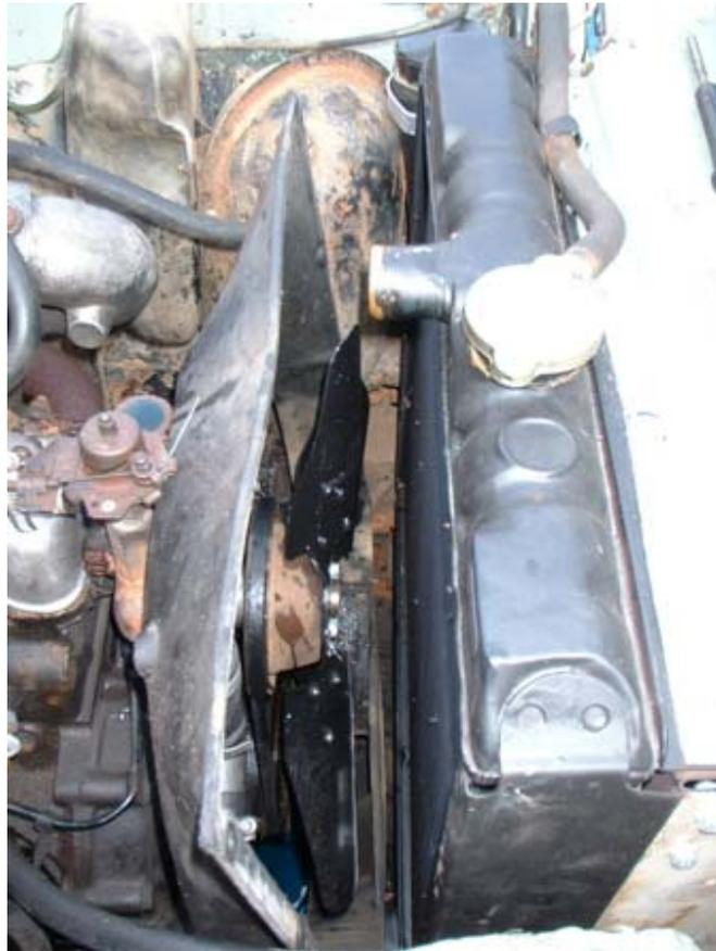
It isn't necessary to remove the radiator to access the pump, now the cowl is pushed back you can get at the four bolts (3/4") holding the fan and pulley assembly to the water pump body. Now you can remove the cowl from the engine bay. And you can also see why they get left off!
