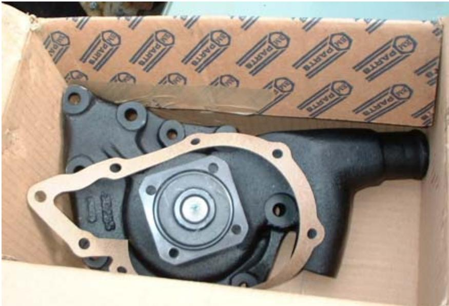
Once the pump is removed from the engine, clean the mating faces,
