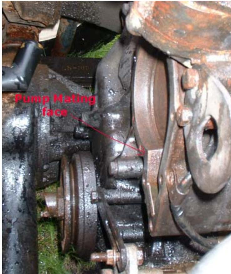
and apply a thin smear of gasket sealant (Hylomar, or Hermetite or similar) and then the gasket. Apply a film of sealant to the pump mating faces, and then fit into position. (You may find it easier to fit the bypass hose to the thermostat housing and slip the pump into it at this point. It's not easy to fit a new hose in there with the pump fitted.) Tighten the bolts.
